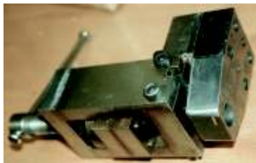
Press for making a holes for output connector
