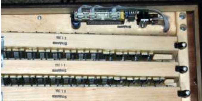
Diatonic accordion right side (without microphone system) Cable through bellow go directly on MIDI processor.
