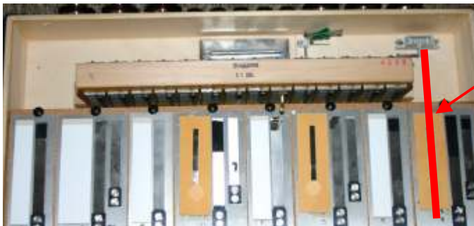
Diatonic accordion left side (without microphone system). The first two reeds are under below fold and cable is over a valve.
