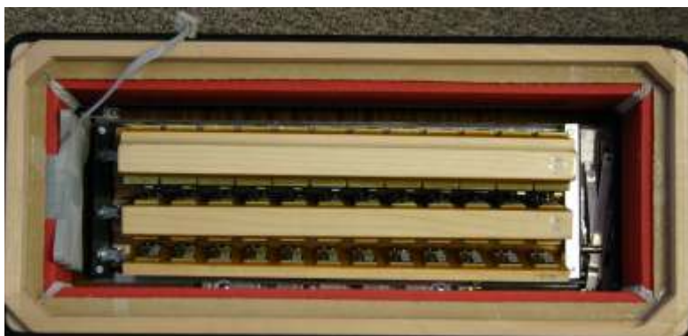
Accordion left side without microphone - only 5 pin bass MIDI cable
